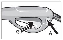
**Step 3** Turn on the pressure washer. Pull trigger to operate unit: Liquid detergent is drawn into the unit and mixed with water. Apply detergent to work area. Do not allow detergent to dry on surface.
